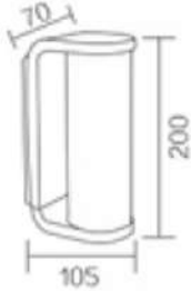
ZN-W202267 Size:105*70*200MM LED Chip:SANAN SMD Wattage:18W CCT:3000K/4000K/6000K
